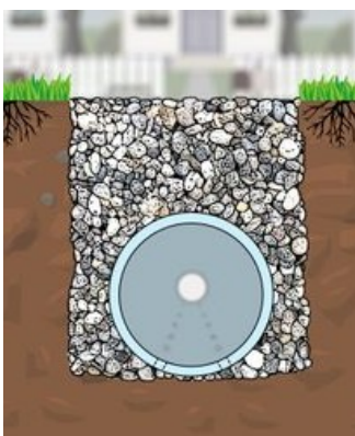
Figure 34: (left) French drain, constructed from a slotted pipe buried in a gravel filled trench. (right) Possible location for a drain, along the grass verge between the road and narrow gauge railway.
